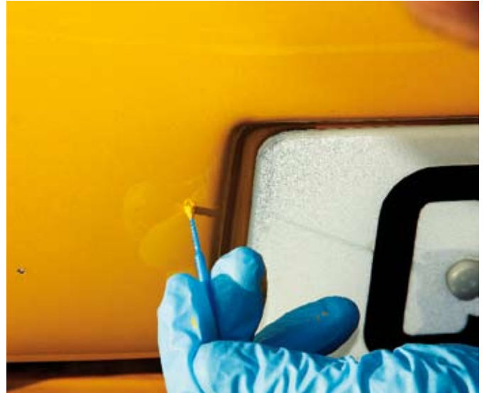
Once you have cleaned the panel, the perfectly matched paint is blobbed into the chip, and dries rapidly – two minutes is all you need for it to set.
